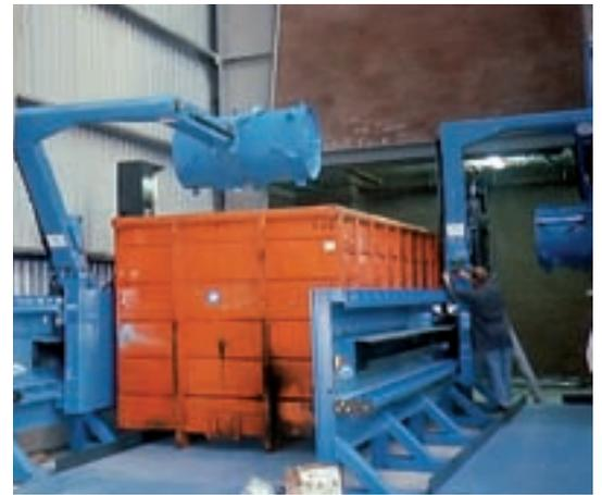
RP 7000 SG (lateral motion) for units with low ceiling height.
